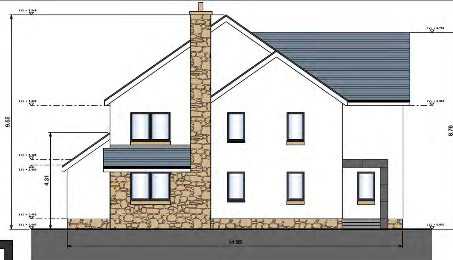
6 House Type A 1:100 Side 1 Elevation
