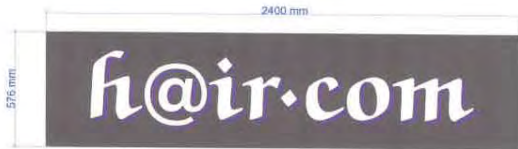
fret cut aluminium composite sign tray with flush to face opal acrylic letters and vinyl graphics rear tray with internal led illumination
