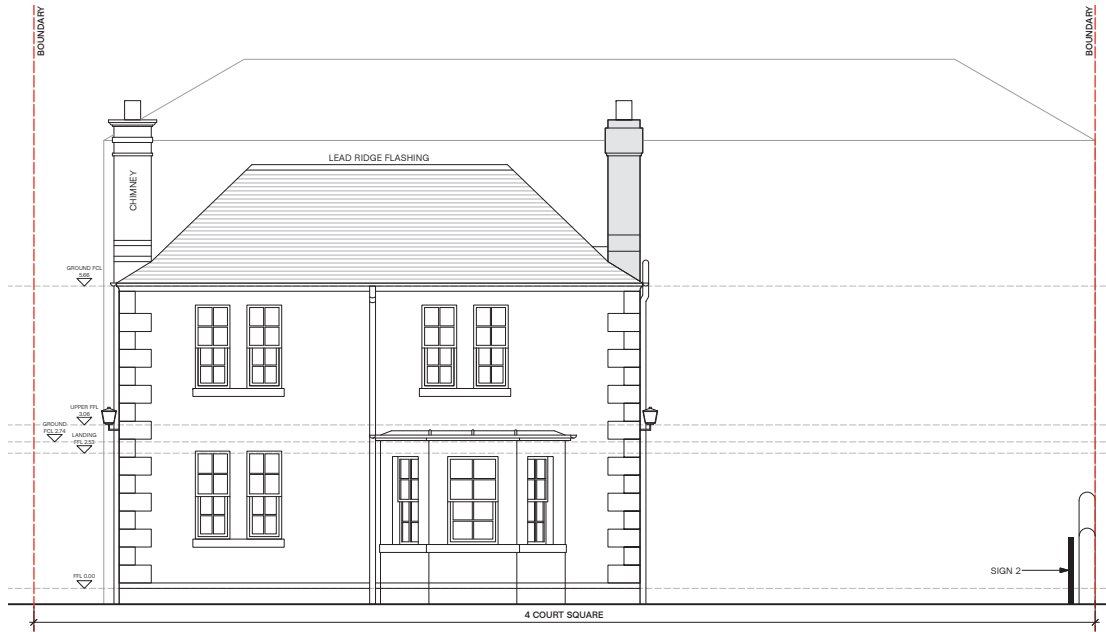
PROPOSED SOUTH ELEVATION FACING STREET / GARAGES 1:50@A1 OR 1:100@A3
