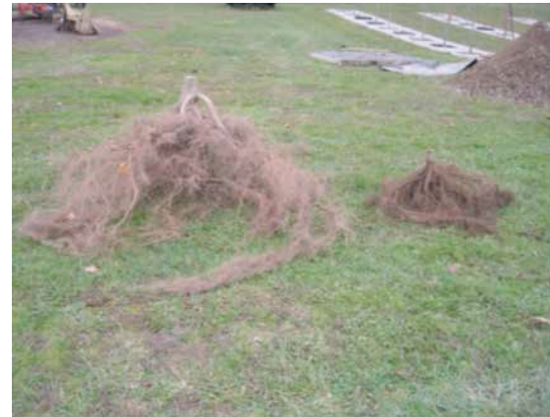
Root system of a tree grown in CU-Structural Soil® (left) compared to one grown in a regular compacted soil (right). Root systems are shown at three years post-transplant.
