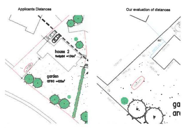
The applicant's site plan shows the distance to the path and not the house. The length to the rear boundary to the house is 12.423m. We believe that the house dimensions and positions should be fixed with clear and accurate dimensions provided to defined reference points.
